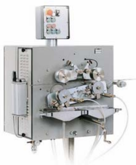
High-speed tandem gravure printing machine from Medek & Schörner
